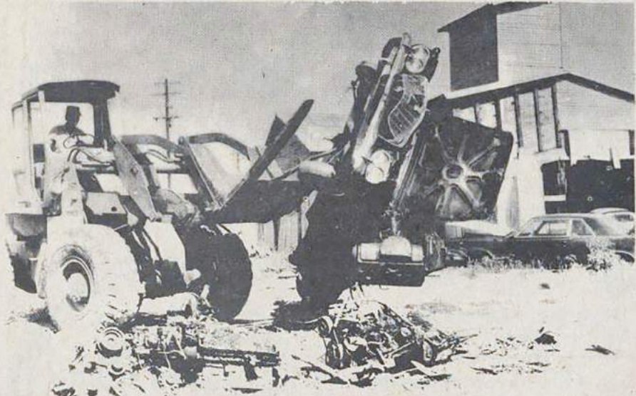
Fork is rammed into engine of auto, knocking it free from car headed for the crusher
